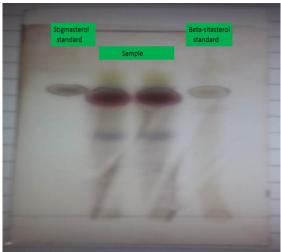
**Figure 3:**TLC of steroid fraction using silica gel GF254nm as adsorbent and S1s as a mobile phase. Visualization by Liebermann-Burchard spray reagent, followed by heating for 10 min at 105°C.
