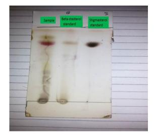
Figure 5:TLC of steroid fraction using silica gel GF254nm as adsorbent and S3s as a mobile phase. Visualization by Liebermann-Burchard spray reagent, followed by heating for 10 min at 105°C.
