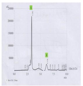
Figure 6: Represent the HPLC analysis of a reference solution mixture containing stagmasterol (0.5 mg/mL) and  $\beta$ sitosterol(0.5mg/mL).
