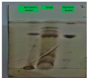
**Figure4:** TLC of steroid fraction using silica gel GF254nm as adsorbent and S2s as a mobile phase. Visualization by Liebermann-Burchard spray reagent, followed by heating for 10 mints at 105°C.
