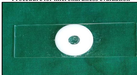
Figure 3: Teflon mould (6mm × 2mm)
