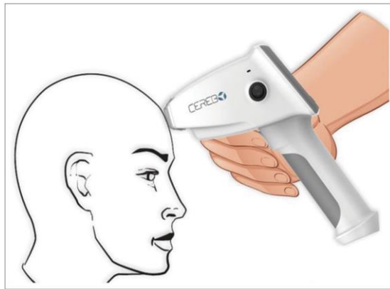
Figure 3: Examination of the left frontal lobe using CEREBO. The device is kept perpendicular to the lobe and then the button is triggered to initiate the scan
