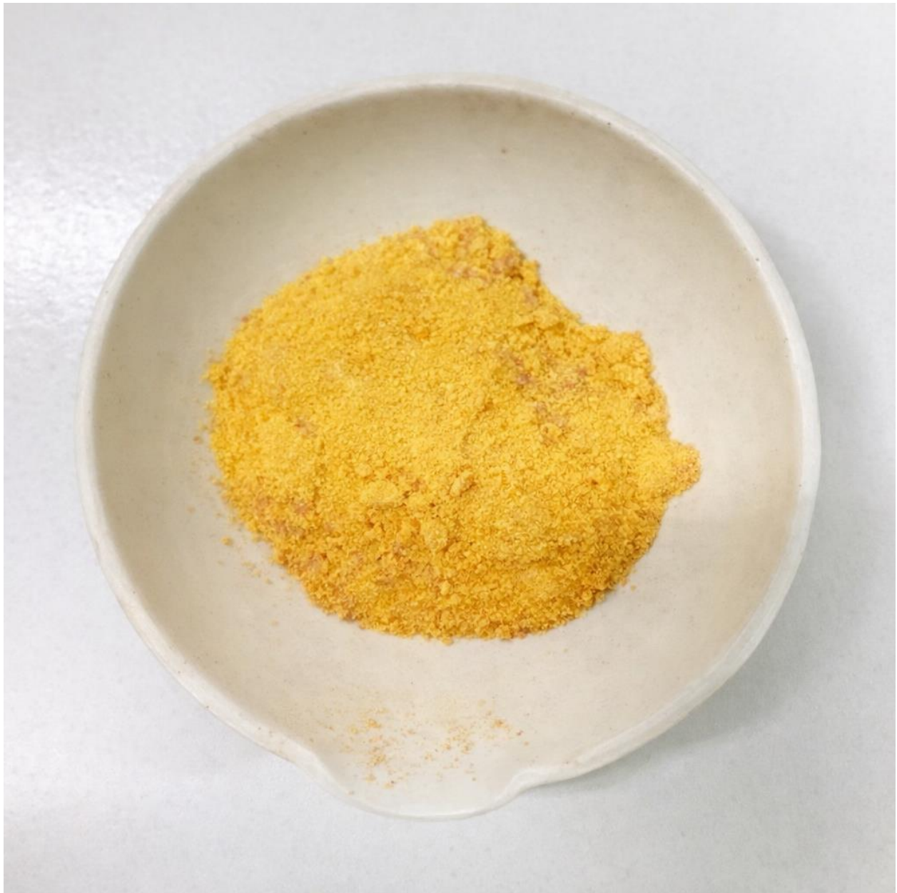
Figure 9. Spray-dried nanosuspension powder of Curcuma xanthorrhiza extract.
